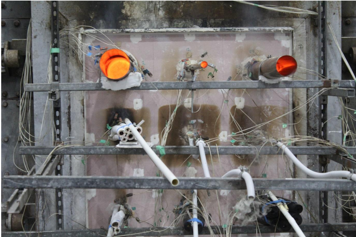
Figure 30 – Unexposed face at 60 minutes
