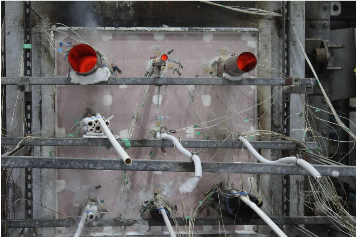
Figure 26 – Unexposed face at 30 minutes
