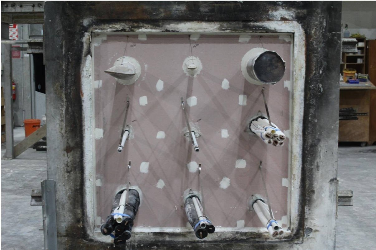
Figure 23 –Exposed face prior to test commencement
